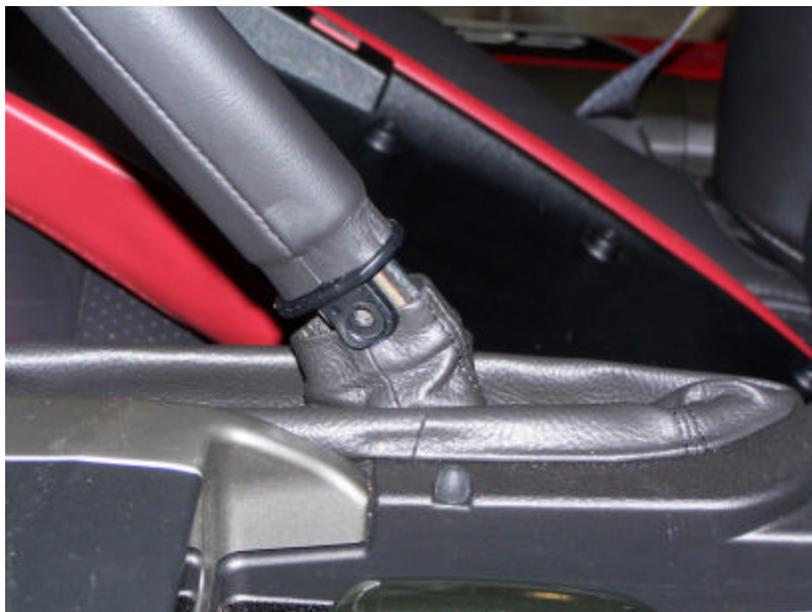
Once you remove the Phillips head screw, the only thing holding the handle in place at this point is the brake release button at the top. The button is held in place with a friction fit and a detent in a notch. To remove (easiest from the passenger side), grip the OEM handle firmly and pull (slide) the handle off which will "pop" the brake release button off the top of the handle. You can now slide the handle off with ease.
