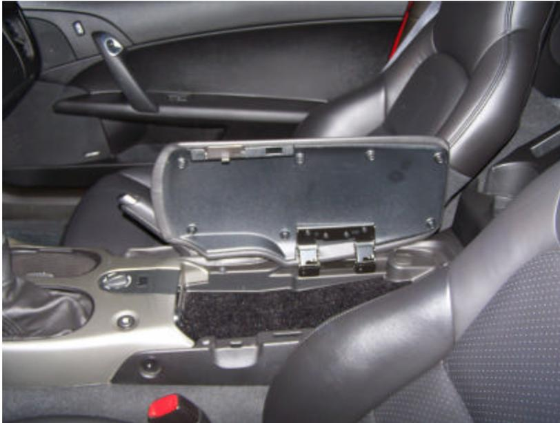
Once the center console cover is off, pull down the e-brake boot to reveal a Phillips head screw which holds the e-brake handle in place.
