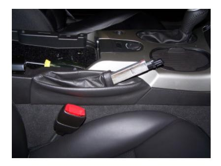
Now that the handle is off you need to remove the OEM brake boot. Take a minute to examine the new Down South Vettes boot. This will give you a better understanding of the four attachment points on the OEM boot.
