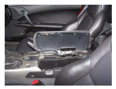
Once the center console cover is off, pull down the e-brake boot to reveal a Phillips head screw which holds the e-brake handle in place.
