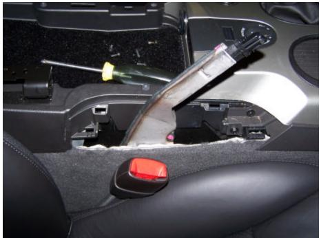
Take the new Down South Vettes brake boot and place it over the top of the handle set at a convenient angle. Through a combination of movements the object is to get the frame and leather boot over the handle and back to level so that you can press it into the four retaining points on the console. Snap everything firmly into place.
