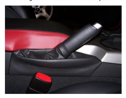
The first step will be to remove the center console cover so you have access to the screw that holds on the e-brake handle. Open the center console to expose 4 T15 Torx screws. Now, remove the center console cover.
