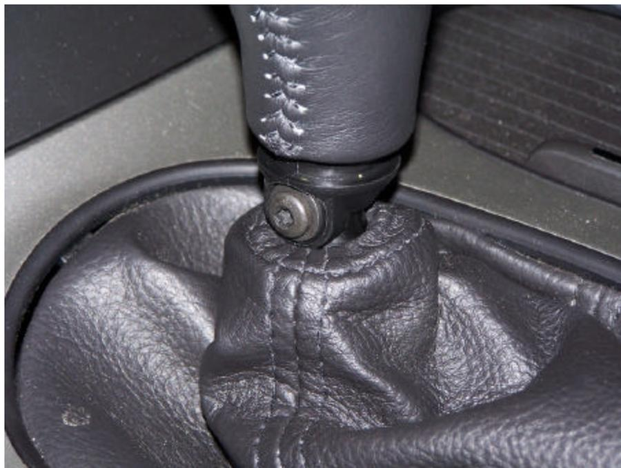
**The Torx screw is seated well and held in place by lock-tite so it will take a little elbow grease to break it free. Remove the screw all the way and the knob will simply lift off.**
