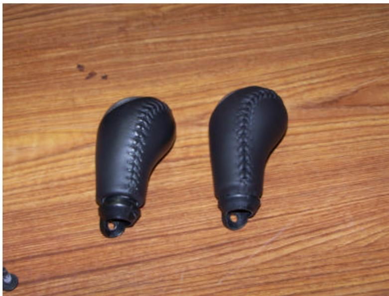
**The shift knob comes off with a T25 torx screw. Just pull down the top of the old boot to expose it.**
