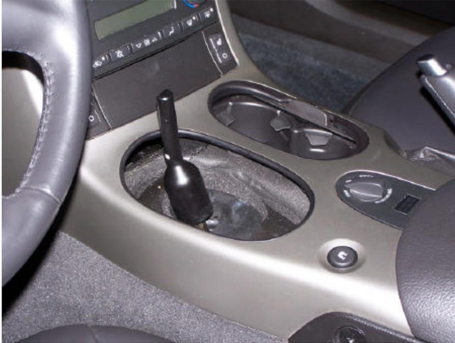
Use your small blade screwdriver to pry up the staples. It is best to put the staple under the boot and pry each side up and off the trim ring. Do this all the way around until all of the staples are free.
