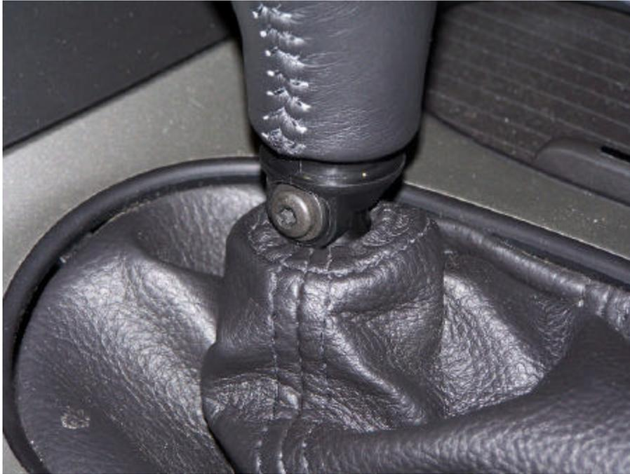
Using your screw driver you will need to pry back the five tabs that hold the trim ring into the console. These are located at roughly 12 o'clock, 2 o'clock, 5 o'clock, 7 o'clock and 10 o'clock.
