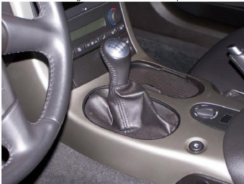
The shift knob comes off with a T25 torx screw. Just pull down the top of the old boot to expose it.
