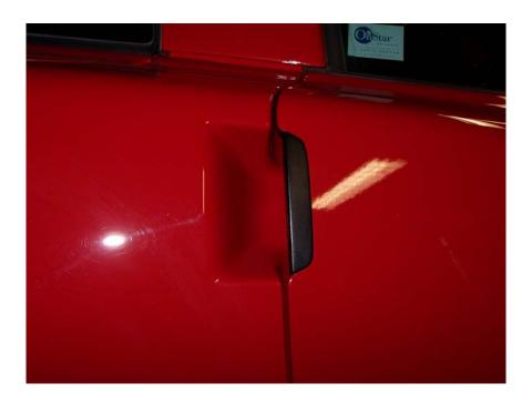
The C6 Corvette door handles are held in place with two Phillips head screws located inside the door jam. You can see them in this photo with the bottom screwed loose and ready to be removed.
