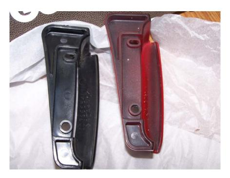
Now the process of putting it all back together. Start by inserting the switch assembly in to the new painted handle. It will likely not fit as snug as it did to the OEM handle and you should get used to how it aligns and fits. You may also find that you need to hold the switch in place during the installation.
