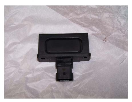
A few will be tempted to leave the switch assembly out of the handle to keep that clean look on the door but I would strongly advise against doing that. The handle is designed to provide support and shock protection for the switch assembly and putting the switch back without the handle will cause the switch to fail somewhere down the road due to the vibration it will face.
