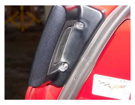
Remove both screws. The handle is a fairly good friction fit to the door panel and it will stay in place once both screws are removed.
