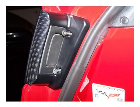
Once both screws are removed you will want to use both hands to work the switch and handle assembly off of the door. Use the thumb and forefinger of your hand to grasp the top and bottom of the switch assembly while using the other hand on the outside of the door to press to slide the switch backwards off the door. The switch and handle assembly will slide straight backward to come off the door. Very little force is required to remove slide the switch.
