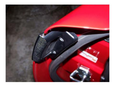
You can pull the assembly off the door and you will find that there is a connector on the back side of the switch. This of course provides the electrical connection for the operation of the door switch.
