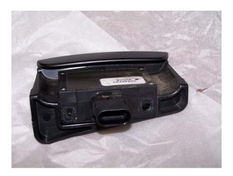
Here is the switch assembly out of the handle.
