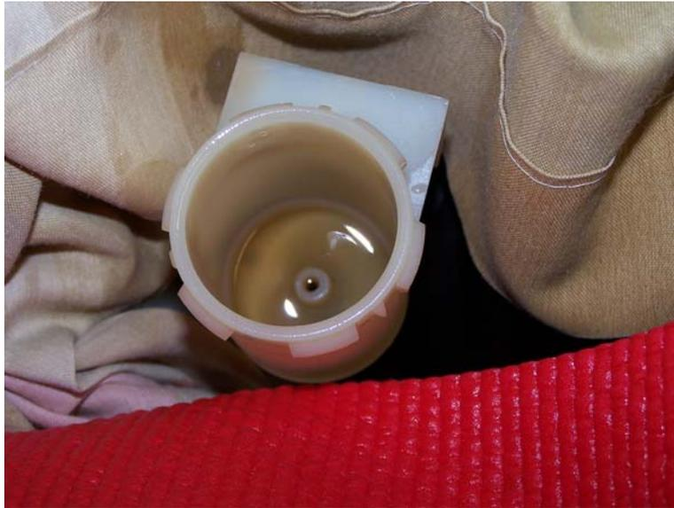
Refill the fluid reservoir with new DOT 4 fluid.
