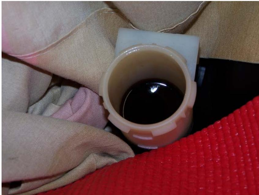
Once you have covered the area, remove the fluid cap from the clutch fluid reservoir. The cap will remove with a quarter turn counter clockwise. The cap also has a rubber bladder that may be drawn down slightly in to the reservoir. This is used to keep air from finding its way in to the clutch system.
