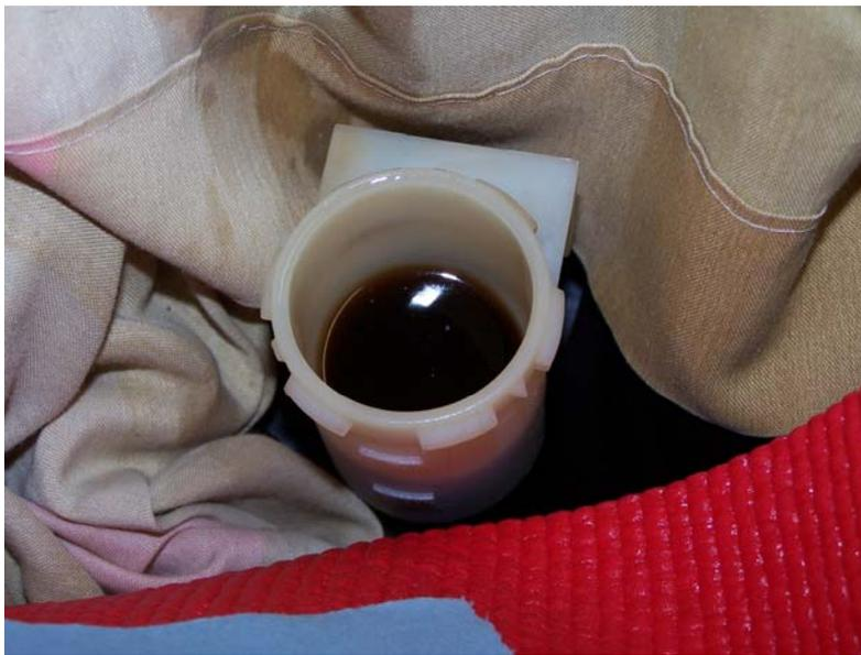
You will need to do this about 10 or so more times before you begin to notice the fluid remaining clear after the clutch pedal is pumped.
