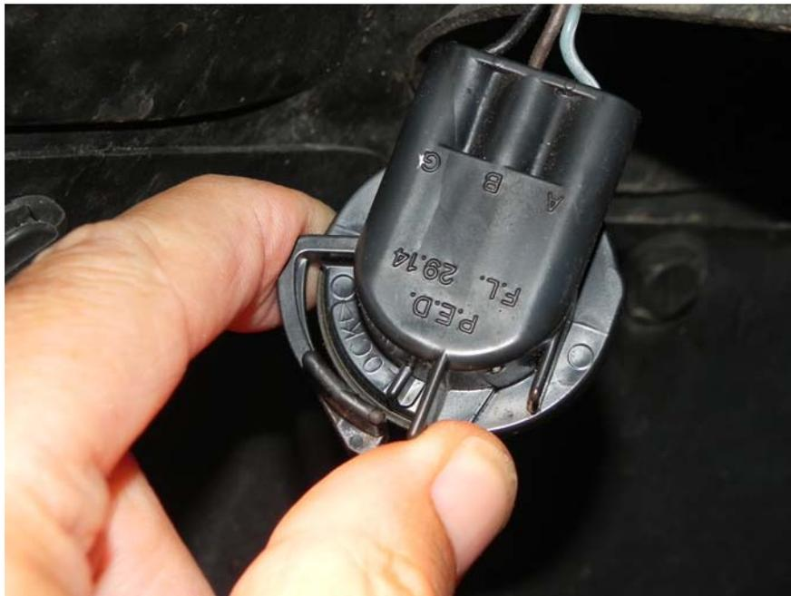
The release will be to the top left of the socket assembly when the socket is installed in the car as the socket will be horizontal and parallel to the ground with the wires off to the right side of the opening.
