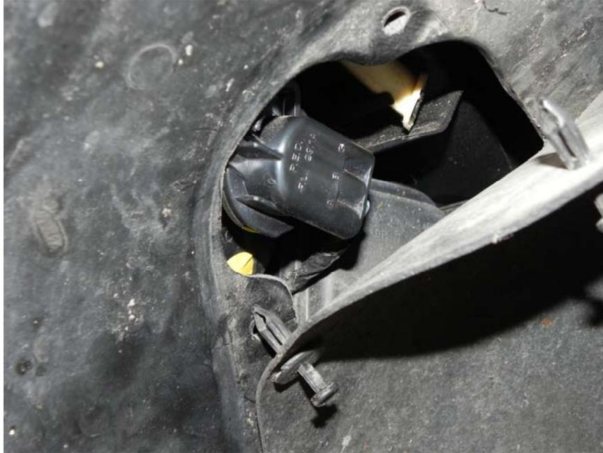
Once the socket is free from the latch you just need to pull (and wiggle) the socket and bulb assembly back out of the opening to get to the bulb. Here is a view of the socket out of the car and a better look at the release that you need to find and press.
