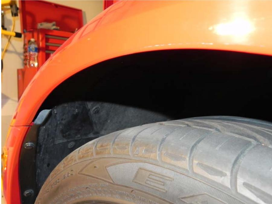
Turning the wheel is your only option if you don't have access to a jack. I would recommend a floor jack for any other change if you have access to one. You don't even need to remove the wheel. If you get the car jacked up off the ground so the top of the wheel is lower than the bottom of the panel you will have plenty of room to get the panel open, twist the socket out and change the bulb.
