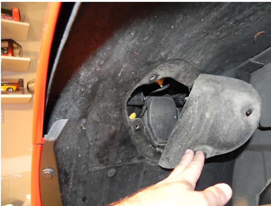
The socket is a twist to lock. There is a release on the top left (about 11:00) as you grasp it with your thumb and forefinger inside the opening. Using your right hand, grasp the socket, find the release and press it down. While holding the release you need to give the socket a quarter turn counter clockwise.
