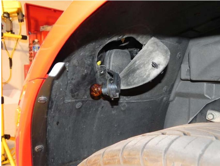
Firmly grasp the bulb and pull it straight out. It is in a location slot in the socket but there is no release or detent that you need to press to remove the bulb from the socket.
